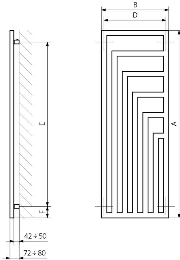
A – Height B – Width C1-C5 – Distance between pipe centres D – Horizontal distance between mounting bracket centres
