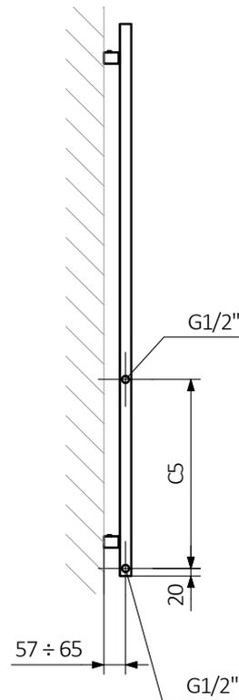
A – Height B – Width C1-C5 – Distance between pipe centres D – Horizontal distance between mounting bracket centres
