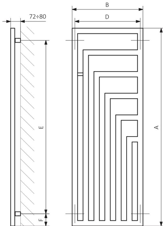
A – Height B – Width C1-C5 – Distance between pipe centres D – Horizontal distance between mounting bracket centres
