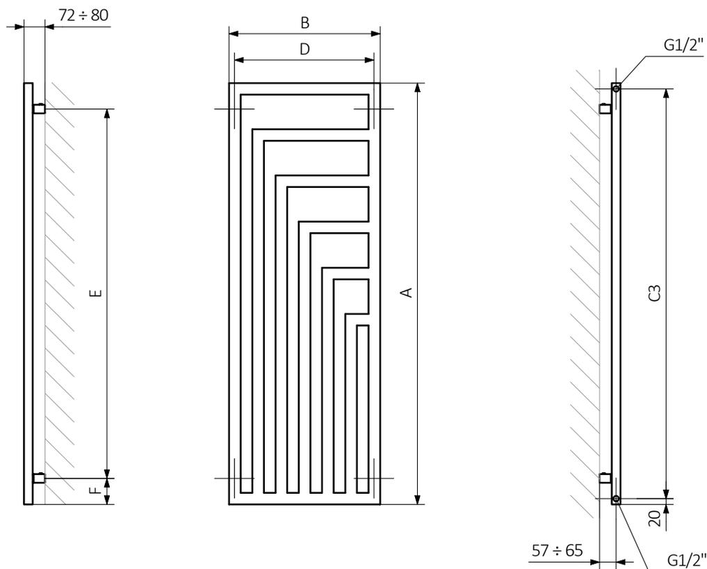
A – Height B – Width C1-C5 – Distance between pipe centres D – Horizontal distance between mounting bracket centres
