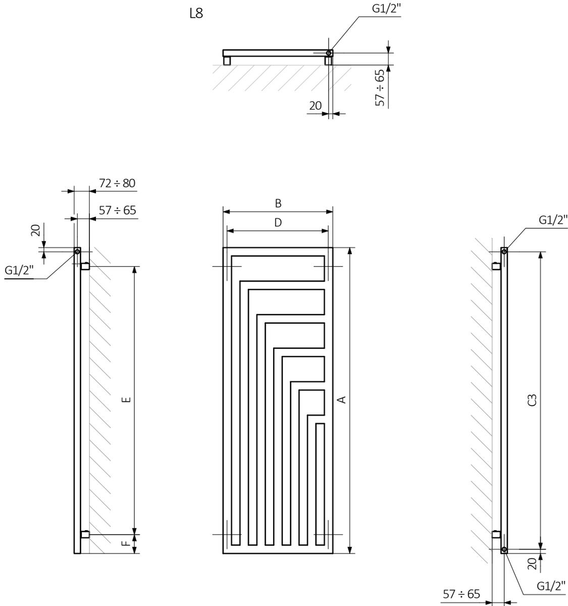
A – Height B – Width C1-C5 – Distance between pipe centres D – Horizontal distance between mounting bracket centres
