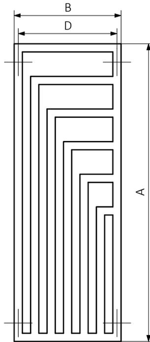
A – Height B – Width C1-C5 – Distance between pipe centres D – Horizontal distance between mounting bracket centres
