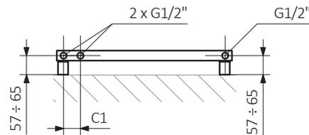
A – Height B – Width C1-C5 – Distance between pipe centres D – Horizontal distance between mounting bracket centres
