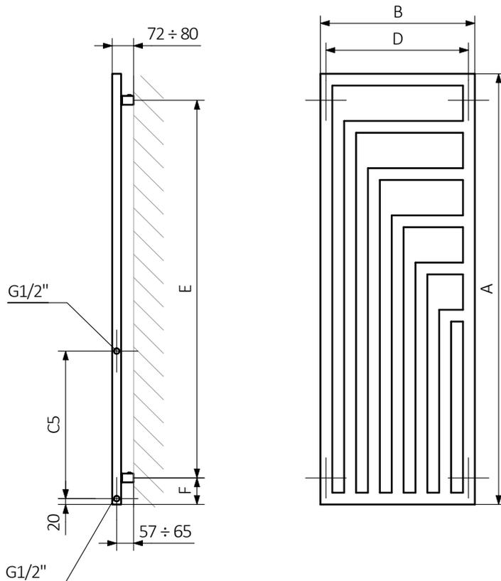
A – Height B – Width C1-C5 – Distance between pipe centres D – Horizontal distance between mounting bracket centres
