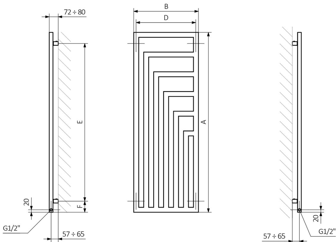
A – Height B – Width C1-C5 – Distance between pipe centres D – Horizontal distance between mounting bracket centres
