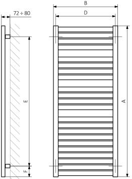
$A-Height \quad B-Width \quad C1-C5-Distance \ between \ pipe \ centres \quad D-Horizontal \ distance \ between \ mounting \ bracket \ centres \\ E-Vertical \ distance \ between \ mounting \ brackets \quad F-Distance \ between \ a \ mounting \ bracket \ and \ the \ bottom \ of \ the \ radiator$
