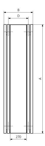
$A-Height\ B-Width\ D-Horizontal\ distance\ between\ mounting\ bracket\ centres\ E-Vertical\ distance\ between\ mounting\ bracket\ shows for the radiator$
