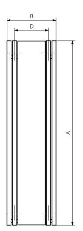
$A-Height\ B-Width\ D-Horizontal\ distance\ between\ mounting\ bracket\ centres\ E-Vertical\ distance\ between\ mounting\ bracket\ shows for the radiator$
