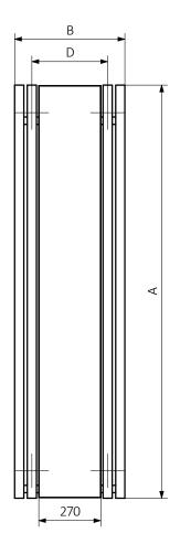
$A-Height\ B-Width\ D-Horizontal\ distance\ between\ mounting\ bracket\ centres\ E-Vertical\ distance\ between\ mounting\ bracket\ shows for the radiator$
