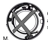
Connection of 100–240 V AC and 12 V DC must not be done simultaneously (Figure M).
