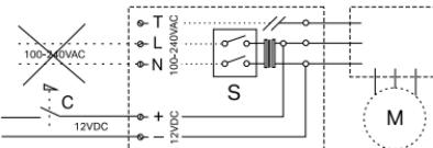
**NB!** For 12VDC always use switches intended for direct current, C.
