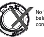
No 100–240 V cables may be laid over the electronics component (Figure N).
