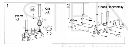
After backfilling the pipe recess, remove the pisitioning plate before tiling.
