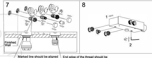
Marked line should be aligned with the finished wall End edge of the thread should be aligned with the finished wall
